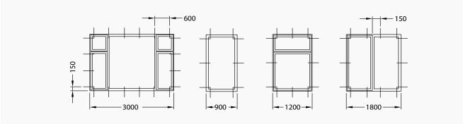
If fixing cleats is the chosen method of installation they should be attached to the outer frame starting at 150mm from the corner and thereafter at a maximum of 600mm centres. The cleats should be screwed into the mainframe in the central reinforcing chamber.
