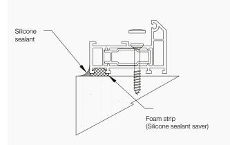
Having manufactured and installed the window so that there is a 5mm gap (approx.) between mainframe and masonry, it may be necessary to insert a flexible foam strip to form a base for the silicone sealant.
